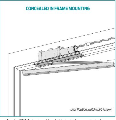
The concealed 2210 Series, heavy duty, high security track closer features complete concealment with special components to minimize tampering and vandalism. Forged steel, single lever arm and heavy steel mounting plate are designed for correctional, vandal prone, institutional, and other high traffic applications. A choice of finishes and cylinder functions meet correctional and vandal resistant requirements.
