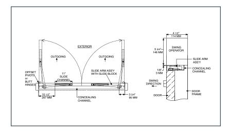
**CONCEALED INDEPENDENT PAIR (OFFSET PIVOT/BUTT HINGE, PUSH) MOUNTING** Offset pivot installations require a bottom pivot and two intermediate pivots.
