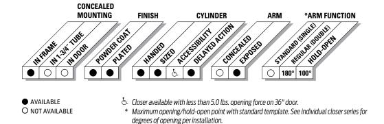
The concealed 5010 Series is a heavy duty closer designed for institutional, high traffic, or other applications exposed to weather or abuse. The double lever arm provides superior door control and a choice of finishes, cylinder functions, and arm functions that meet virtually all architectural requirements.
